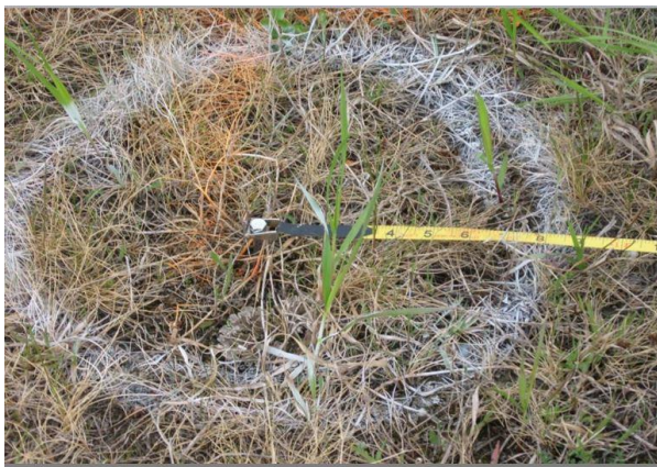
Measuring from pipe to pipe across the runway Bolt holds tape measure in reference marker.
