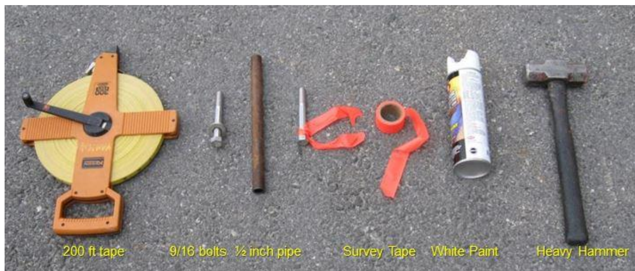
Figure B-4. Tools used to install permanent markings reference points.
