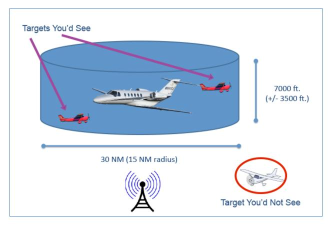
ADS-B Out requires a transmitter. However, the FCC and FAA only allow transmitters on certified systems. The FAA does not allow any portable system (like one connected to an iPad) to be certified. Thus, it is impossible to purchase a portable ADS-B Out system; you must purchase a much more expensive certified system and have it installed in your plane to get ADS-B Out.
