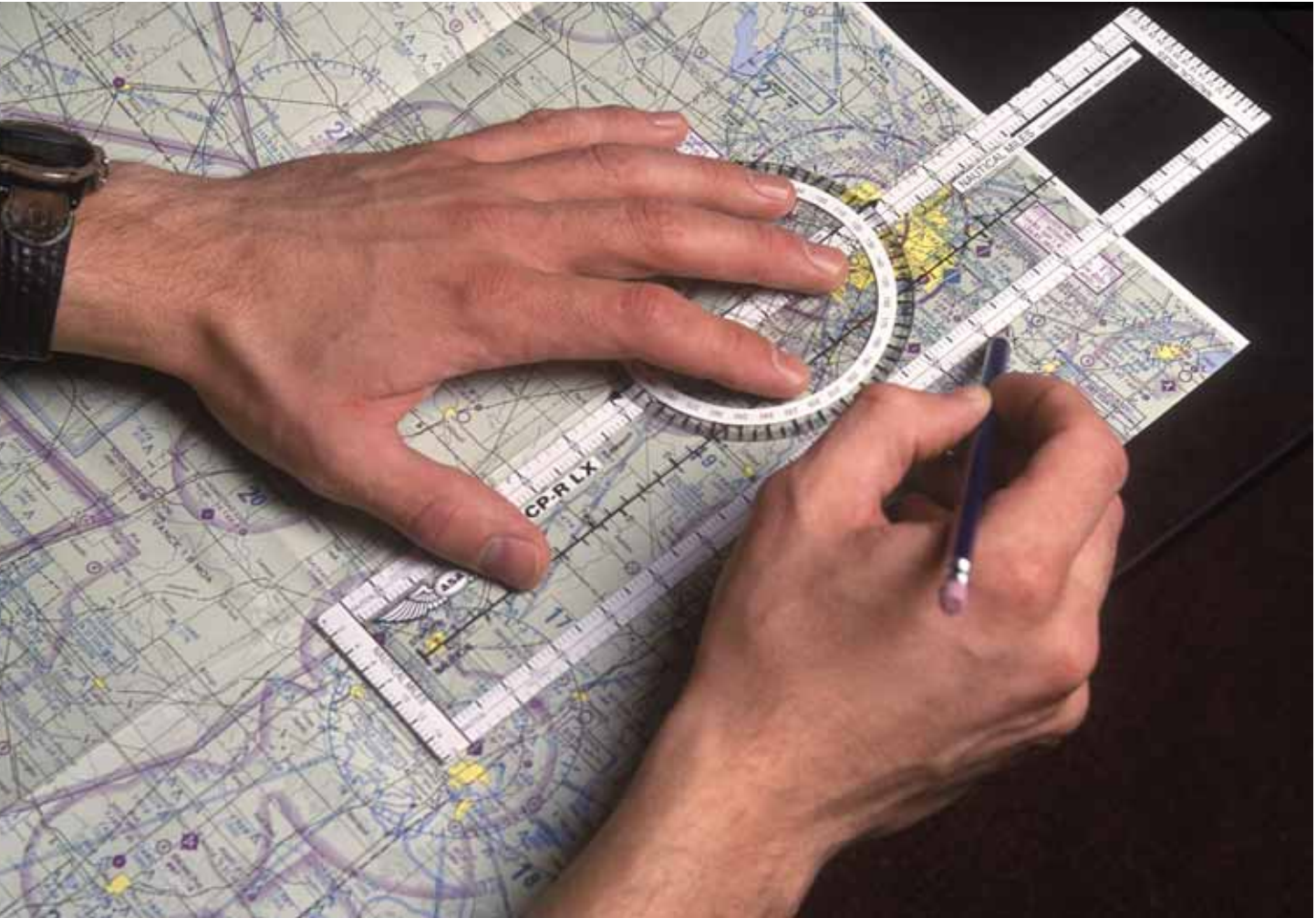
A student pilot uses an aeronautical ruler to mark a flight path.
