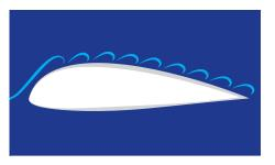
SMOOTH BOUNDARY LAYER AIRFLOW OVER AIRFOILS IS CRITICAL TO SAFE FLIGHT— DEGRADE IT WITH ANY SNOW, FROST, OR ICE AND FLIGHT MAY NOT HAPPEN.
