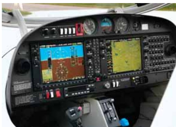
New TAA Instrument panel in a Diamond DA-40.
