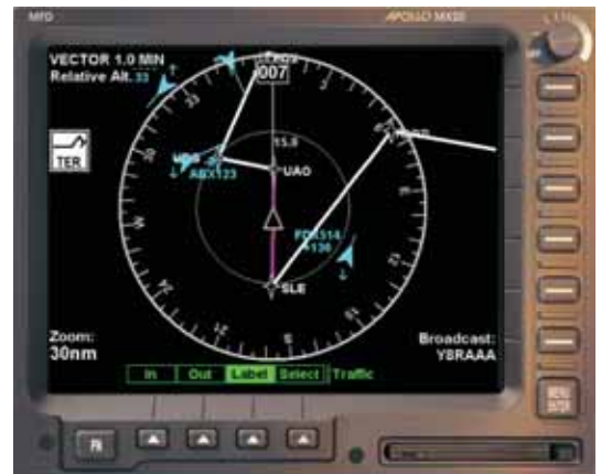
Traffic displayed on an Apollo MX20 (below).
