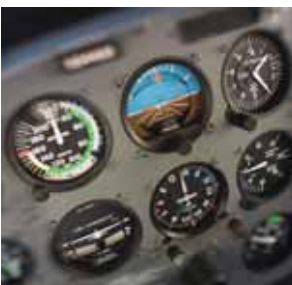
Traditional "steam gauges" or "six-pack" on an instrument panel (below).
