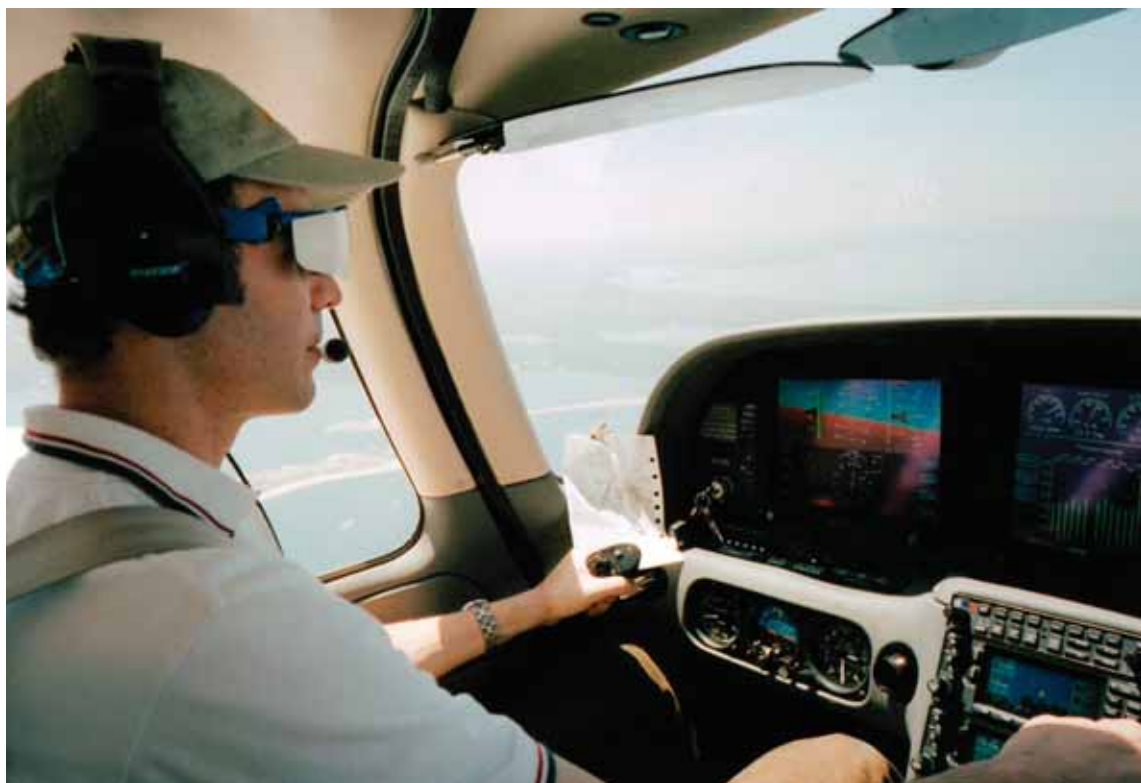
Instrument training in a Cirrus model aircraft (note the back-up instruments in front of the pilot, under the PFD).
