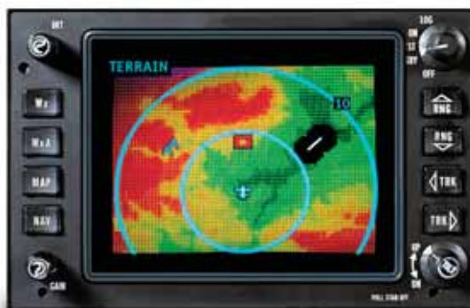
TAWS-B units are most commonly installed in general aviation aircraft.
