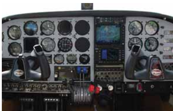
Retro TAA Instrument panel in a Piper Twin Comanche.
