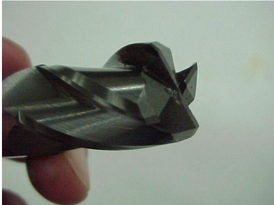
FIGURE 4 END MILL FOR SPOT FACING PROPELLER FLANGE FRONT FACE
