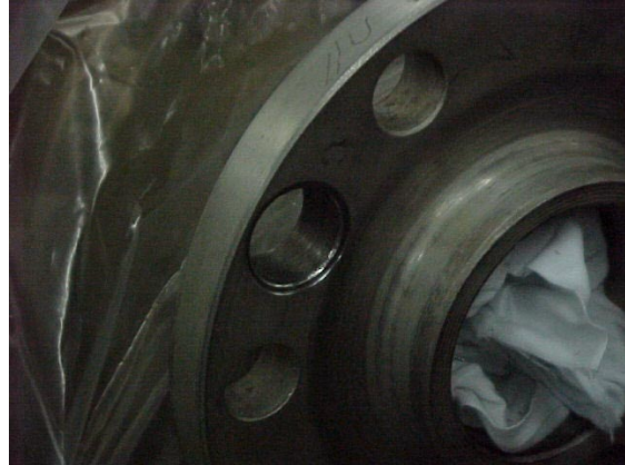
FIGURE 12 CORE SAMPLE HOLE AFTER CHAMFERING
