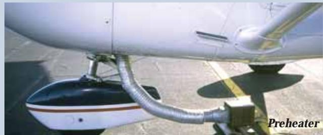
When using a hot-air preheater, plug the air intakes on either side of the propeller, and place a blanket over the cowling to contain the heated air. Preheat for 15 to 20 minutes to ensure even heating for the entire engine.
