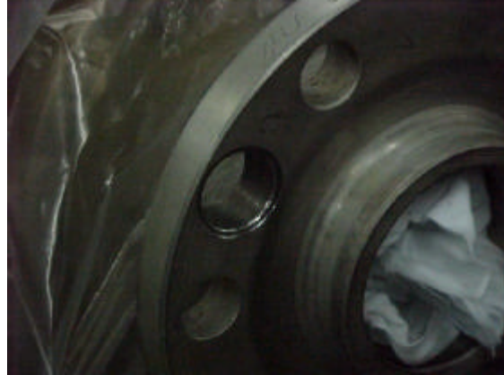
FIGURE 12 CORE SAMPLE HOLE AFTER CHAMFERING
