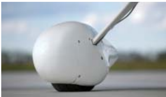
A new speed kit includes smaller tires (right), more tightly enclosed wheels, and streamlined struts.
