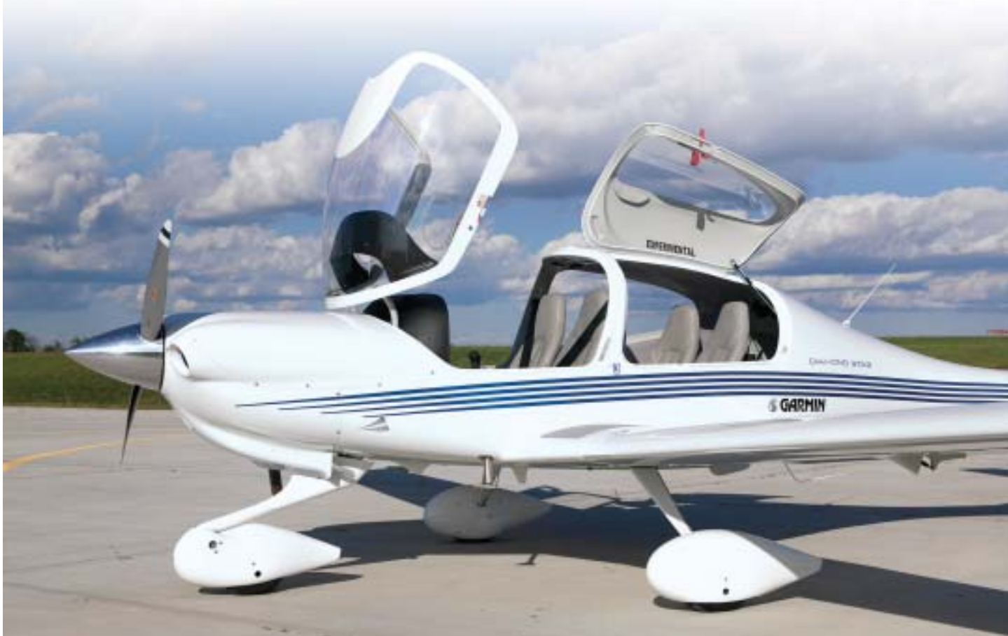
A new speed kit includes smaller tires (right), more tightly enclosed wheels, and streamlined struts.
