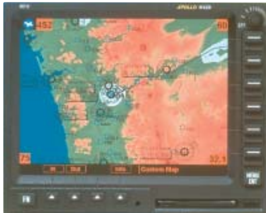
Cockpit display of traffic information (CDTI) shows uplinked targets from ATC radar (above). Blue symbols indicate conflicting traffic location, relative altitude, and flight paths. UPSAT's MX20 used in the Capstone project has a terrain and navaid database to boost situational awareness (right).
