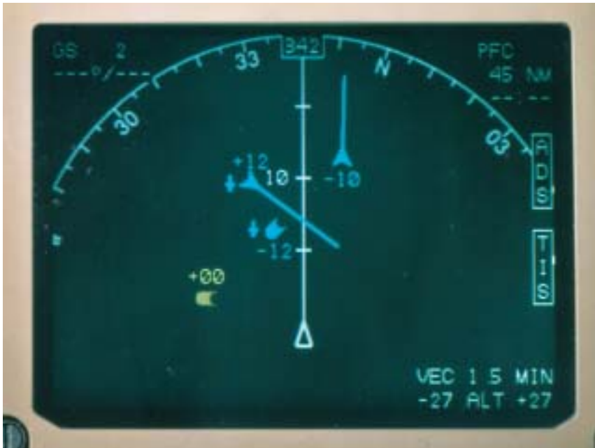
Cockpit display of traffic information (CDTI) shows uplinked targets from ATC radar (above). Blue symbols indicate conflicting traffic location, relative altitude, and flight paths. UPSAT's MX20 used in the Capstone project has a terrain and navaid database to boost situational awareness (right).
