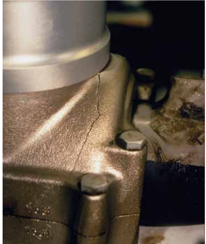
A cracked hub
