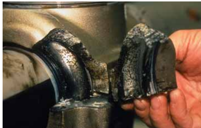
A cracked aluminum hub
