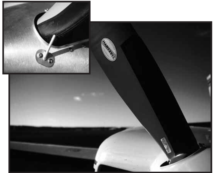
Alcohol (inset) and electrically heated prop anti-ice equipment
