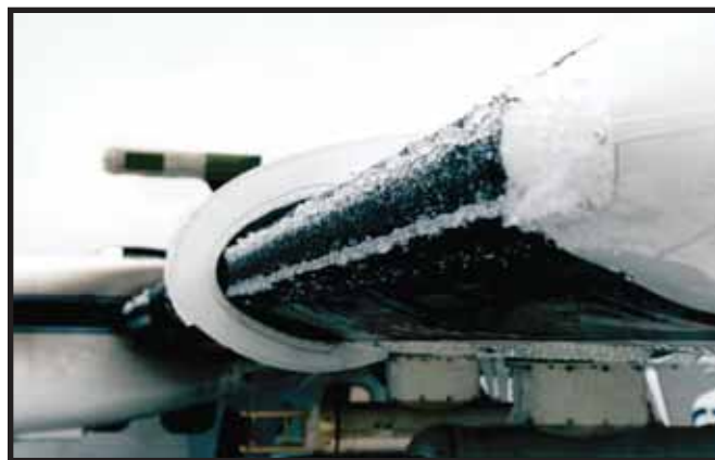
Clear ice formation on wing leading edge
