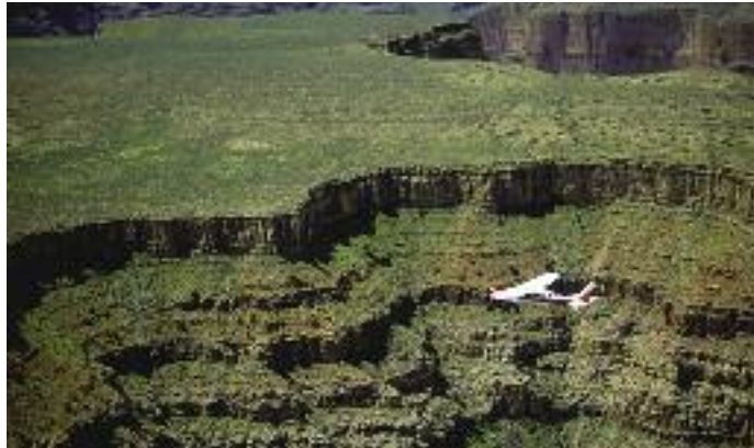
Density altitude can be deceiving, and many canyons are not like the Grand Canyon. Even if the terrain climbs only slightly faster than the aircraft, a sudden stop may be inevitable.
