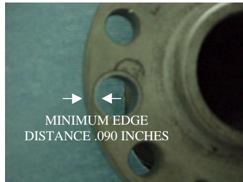
FIGURE 13 CORE SAMPLE HOLE MINIMUM EDGE DISTANCE
