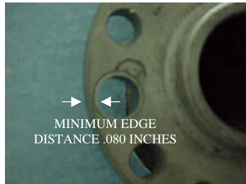
FIGURE 13 CORE SAMPLE HOLE MINIMUM EDGE DISTANCE
