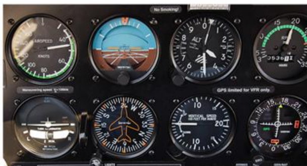
A TYPICAL INSTRUMENT DISPLAY DURING SLOW FLIGHT —notice the power setting, which is usually around 2,000 rpm in single-engine trainers.
