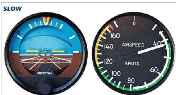
SLOW FLIGHT—ALSO CALLED MINIMUM CONTROLLABLE AIRSPEED —requires a nose-high attitude to maintain altitude at the slow airspeed (above).
