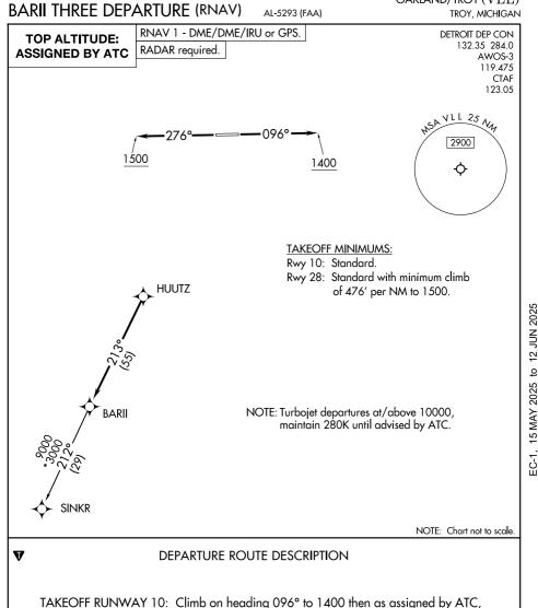
TAKEOFF RUNWAY 10: Climb on heading 096° to 1400 then as assigned by ATC, thence....
