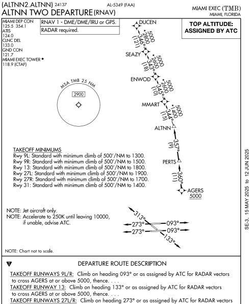
to cross AGERS at or above 5000, thence. . . TAKEOFF RUNWAY 31: Climb on heading 313° or as assigned by ATC for RADAR vectors to cross AGERS at or above 5000, thence. . . .
