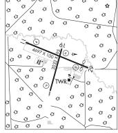
removal equipment oprs monitor CTAF when twr clsd. Supplementary lgtd windcones Rwy 11 and Rwy 01. Rapidly rising terrain 1 NM northwest to northeast of arpt. R6901B 500 yds dep end Rwy 11. Controlled small arms range 1,000 yds dep end Rwy 19. Rwy 01 and 11-29, NSTD safety area byd each end due to terrain grade and fencing. NSTD north lateral clearance Rwy 11-29: See KCMY AP/1 for further information. Rwy 11 dep be alert for optical illusion, vehicles on road may appear to be on rwy.
