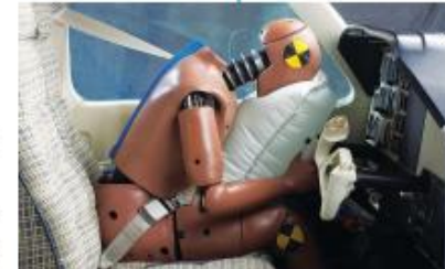
AmSafe's Seatbelt Airbag System (SOARS) is an example of an aftermarket lapbelt airbag restraint system, which is designed to mitigate head and torso injury in aircraft crash conditions. Photo courtesy AmSafe, Inc.
